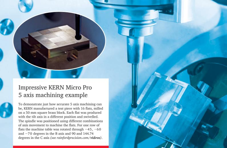
The results show all the surfaces produced in the row have only deviated by +/-0.0005 mm and all 16 surfaces are flat to within 0.0023 mm, *impressive* accurate machining.
