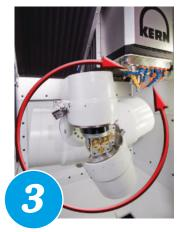
2 axis table with 280° swivel. The 2-axis table has a swivelling range of  $\pm 110^\circ$  (with an option of  $-170^\circ$  to  $+110^\circ$  giving a total 280°). The extra capability is very useful to remove swarf from pockets prior to machining with small diameter cutters.
