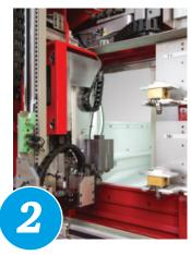
Simple Automation (option) For customers with small component sizes and small batch sizes the 30 position integral magazine will be very attractive, this unit fits under the tool magazine pallets and can change workpieces up to  $70 \times 70 \times 150$  mm high.
