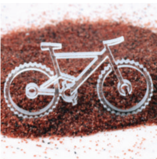
Decorative glass bike: Machined from 3 mm plate glass showing details on tyres and wheel axles.
